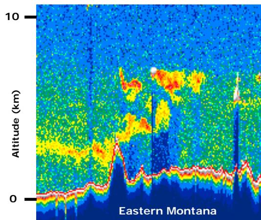
**Figure 4:** 532 nm backscatter return signal from the CALIPSO lidar, taken at 3:20 AM local time on July 31, 2007. The satellite data show the vertical distribution of fine particles over eastern Montana from the wildfires on July 30, 2007. The red and yellow areas indicate elevated particulate concentrations.
