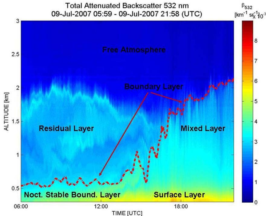
**Figure 2.** UMBC ELF 532 nm total attenuated backscatter ( $\beta_{532}$ ) timeseries plot for July 9, 2007. The red line represents the height of the planetary boundary layer during the course of the day.
