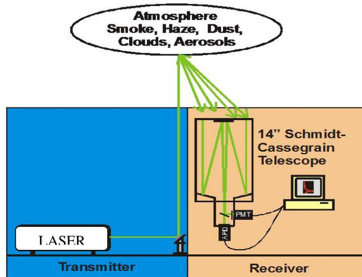
Figure 1. The basic components of a lidar system.
